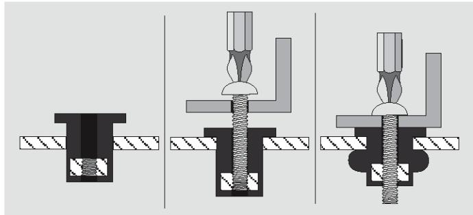
1. Place Well-Nut insert all the way into pre-drilled hole until flange is firmly against mounting surface.
