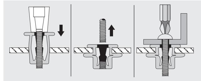
1. Thread JACK NUT insert onto mandrel of installation tool, then insert all the way into predrilled hole until flange is firmly against mounting surface.
